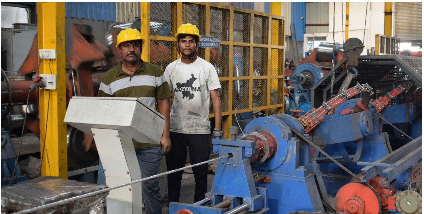
Stranding machine in the conductor hall
