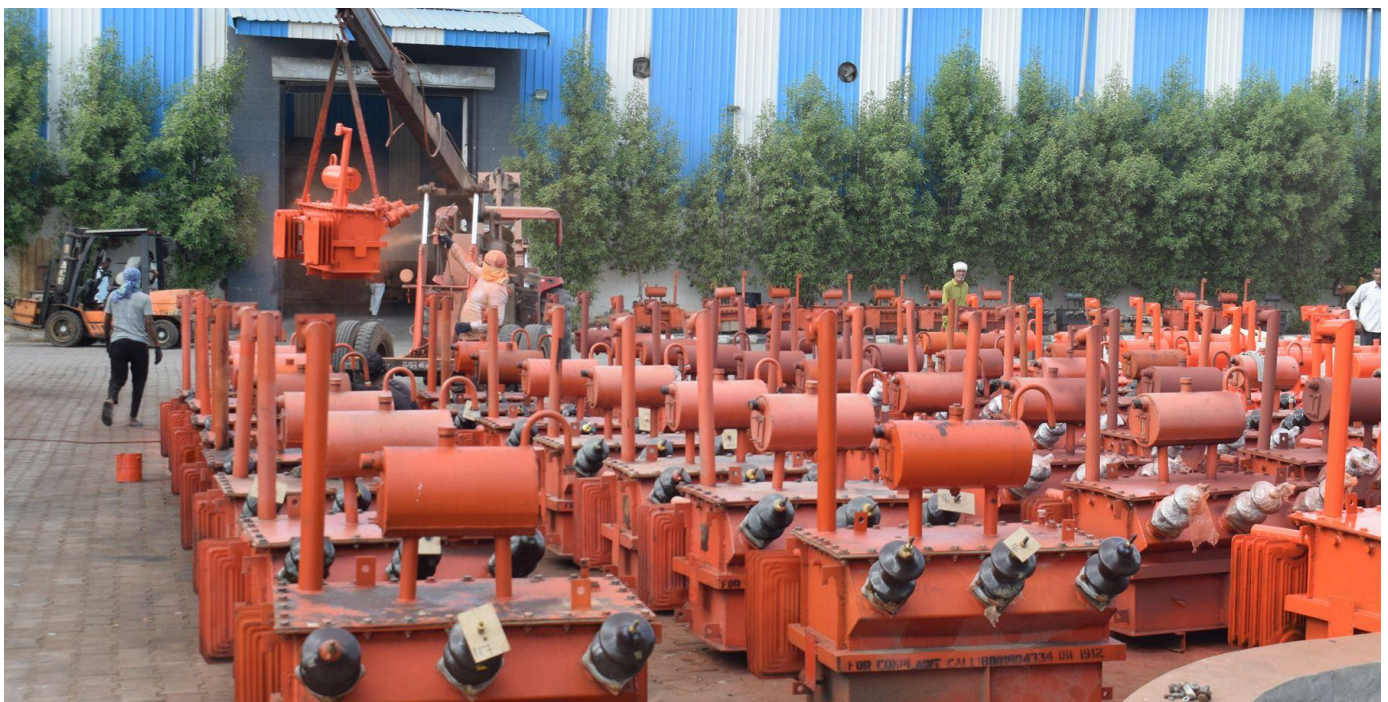
Finished distribution transformers in the dispatch yard
