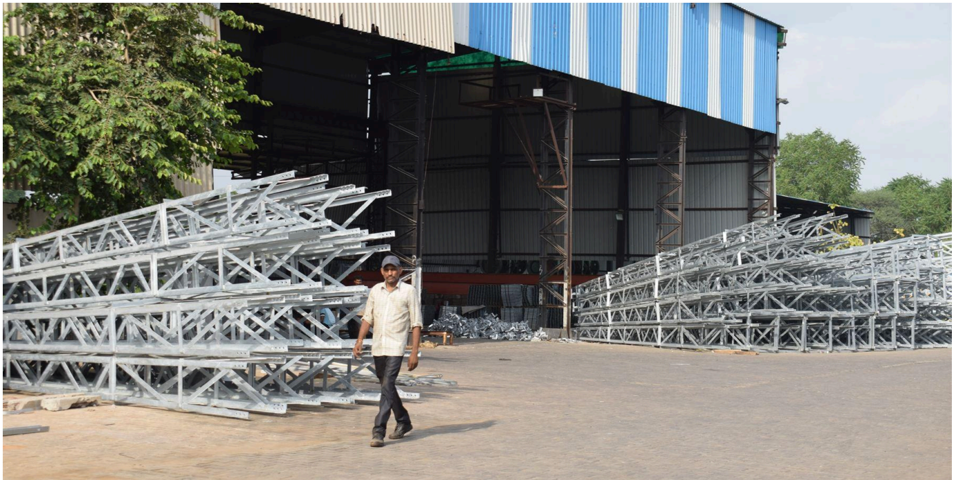
Galvanized tower sections leaving the shed
