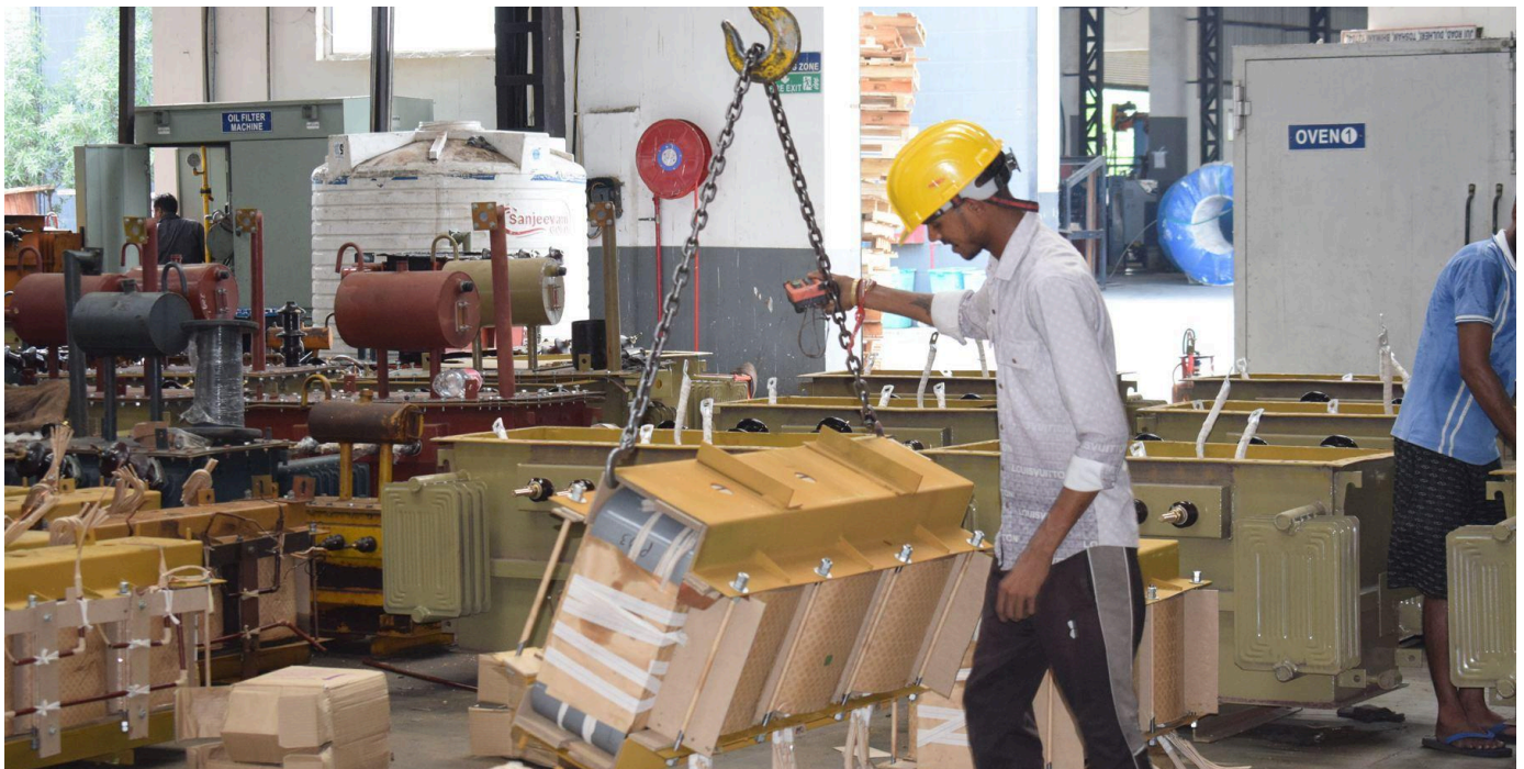
Core-and-coil assembly bay
