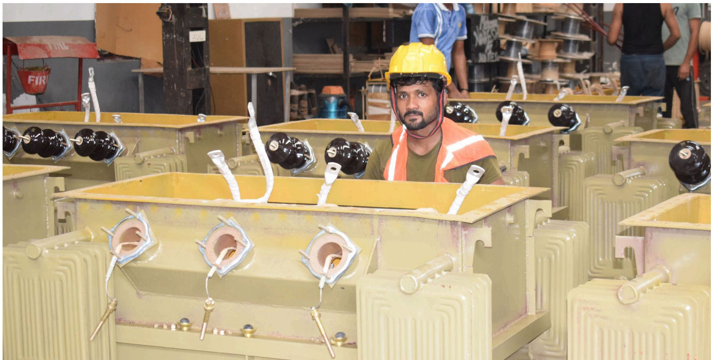
Tanks awaiting core-and-coil assembly
